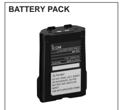
BP-245 7.4V/2000mAh Li-Ion battery pack. Provides 15–16 hours* operating time (approx.). Same as supplied. *(Tx (Hi): Rx: standby=5:5:90).
